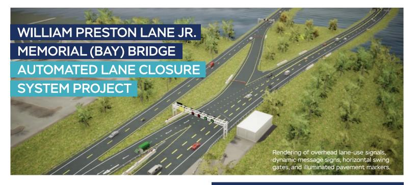
The Bay Bridge automated lane closure system (ALCS) is a project constructed for opening and closing lanes for two-way traffic operations on the bridge. Since two-way operations were implemented, lane closures have been done manually. The ALCS will enhance the current manual system for motorists by allowing maintenance crews to remotely implement and discontinue two-way traffic on the Bay Bridge's Eastern and Western Shores.
