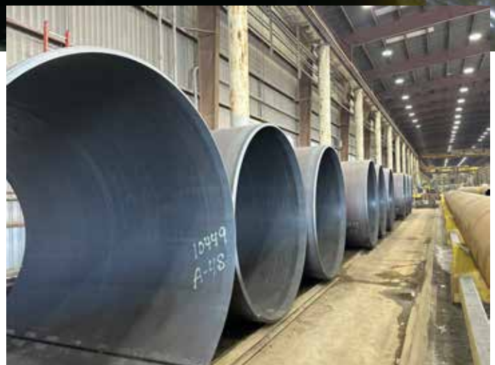
Test pile fabrication.
