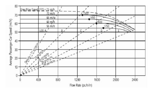
Based on the established speed-traffic flow relationships and in order to guarantee that managed lanes almost always operate in stable and free flowing traffic, we propose that the traffic flow threshold is set at 1,450 PCE vehicles per hour per lane (assuming managed lanes posted speeds are set to 65 mph).
