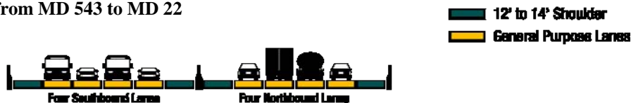
Figure 6 – Preliminary General Purpose Lanes Alternate - Typical Roadway Section
